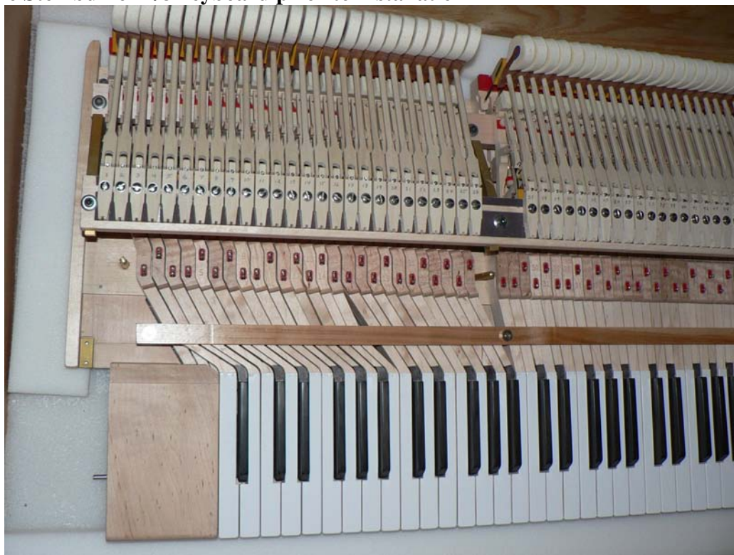
The Steinbuhler 7/8 keyboard prior to installation
